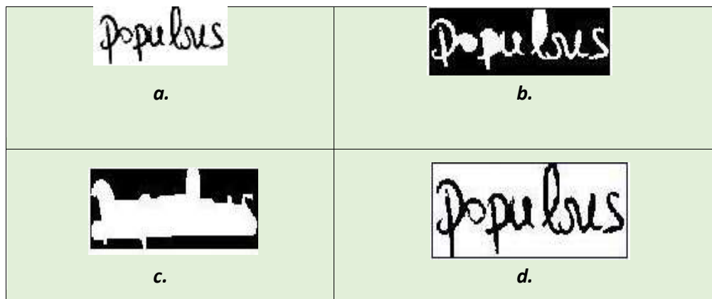
Figure 14 - Overview of Segmentation Process: (a) Original Image (b) Filling of holes (c) RLSA (d) Segmented word
