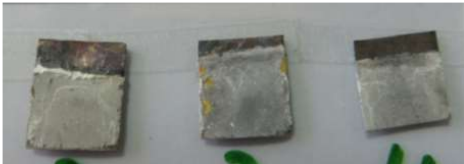
Figure 5-4 The coating containing ZnO nanostructures after Annealing in Air.
