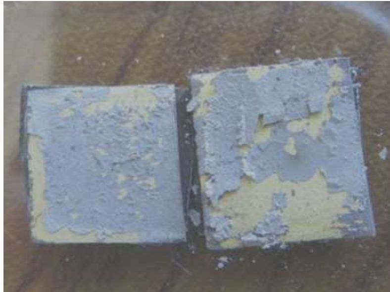
Figure 5-3 The coating containing ZnO nanostructures after Annealing in Ar environment.
