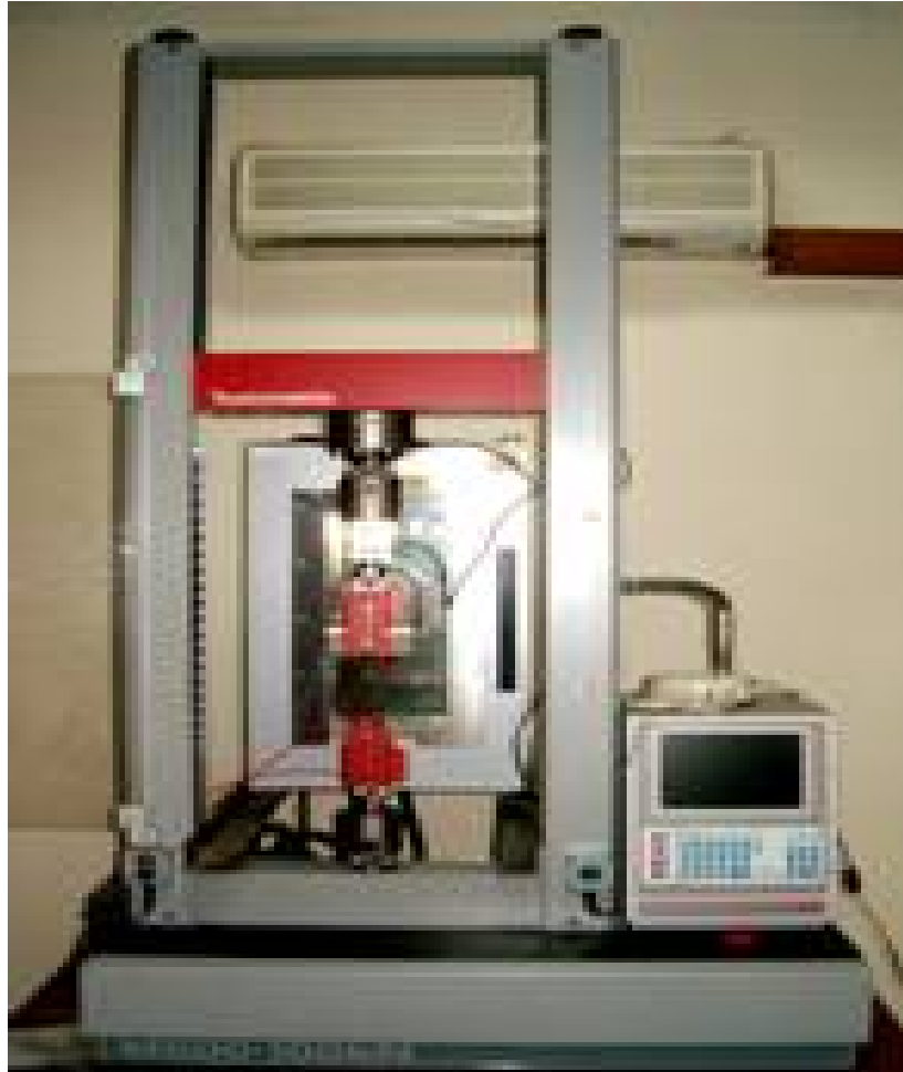
Universal Testing Machine (UTM), Testometric Inc. UK,
