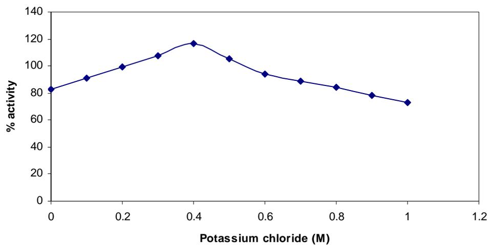
**Fig. 4.42 Effect of potassium chloride on the stability of mutant derived enzyme**
