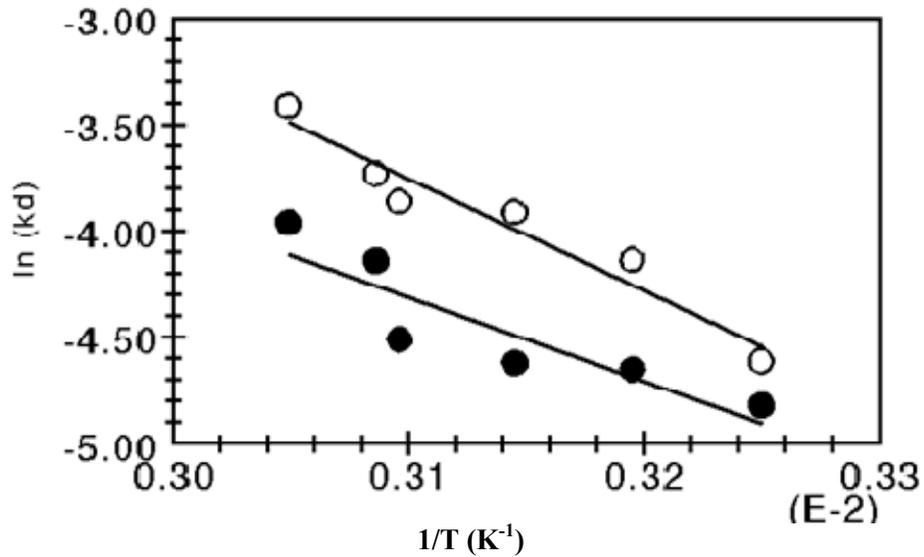
Fig. 4.36 Arrhenius plot to determine the activation energy for deactivation of urate oxidase derived from the parental and mutant derived strain.
